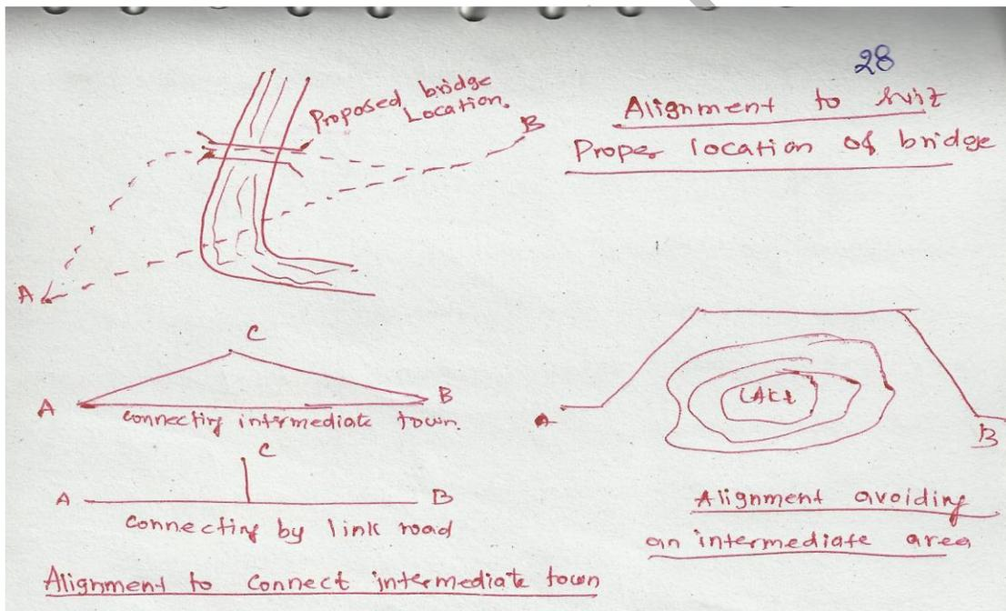
In fig.2.shows that the straight alignment between stations A and B which passes across the river band is to be deviated along the path shown in order to cross the river at a proper bridge location.
