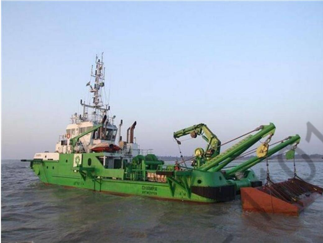
Often used for environmentally sensitive projects, water injection dredgers work by fluidizing the material by pumping water into the bed material. Once it is fluidized it is either moved by a second burst of water or is carried away by the natural current.
