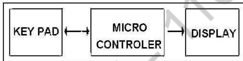
**Interfacing Keyboard to 8051 Microcontroller**
