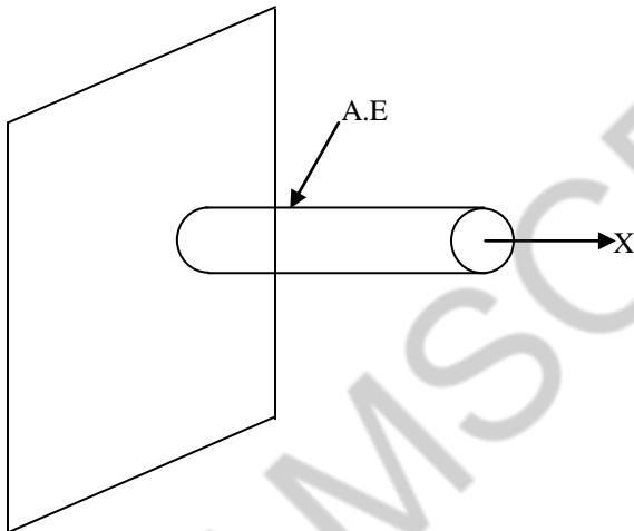
Consider a uniform cross – section bar (Figure) of length L of a material whose Young's modulus and density are given by E and  $\rho$ . Estimate the natural frequencies of axial vibration of the are using both consistent and lumped mass matrices.
