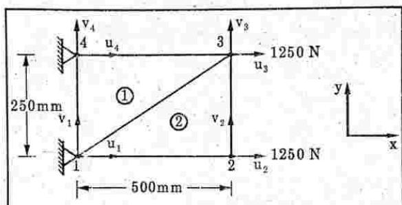
**For element (1):** [Nodal displacements are  $u_1$   $v_2$ ,  $u_3$   $v_3$  and  $u_4$   $v_4$ ]
