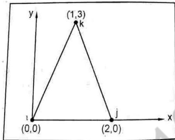
**Fig. 7 Triangular elastic elements**
