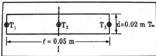
**To find:** Temperature at the midpoint of the rod ( $T_2$ )
