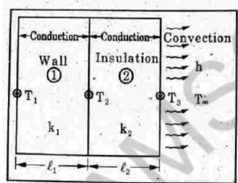
$$\frac{A_1 k_1}{\ell_1} \begin{bmatrix} 1 & -1 \\ -1 & 1 \end{bmatrix} \begin{Bmatrix} T_1 \\ T_2 \end{Bmatrix} = \begin{Bmatrix} F_1 \\ F_2 \end{Bmatrix}$$
